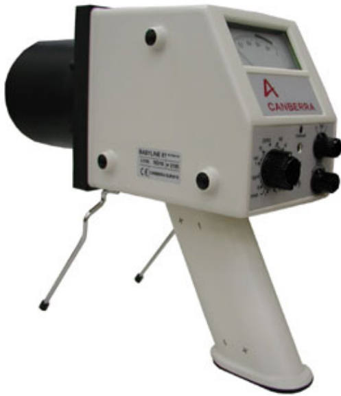
Babyline for measuring the absorbed dose of \gamma photons with hood (eye lens equivalent dose) and X, \gamma and \beta - without the hood (skin equivalent dose).
